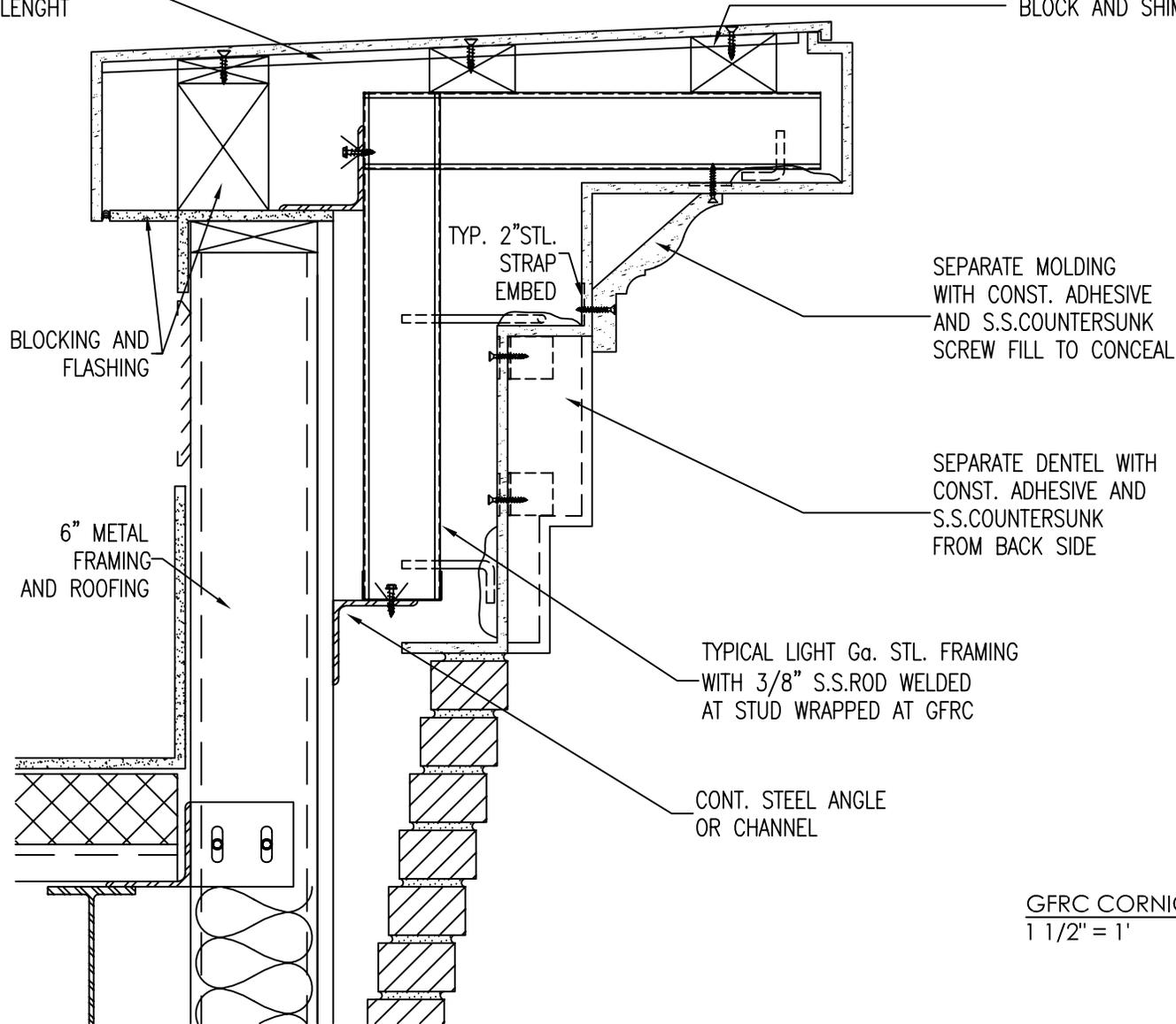
SEPARATE MOLDING WITH CONST. ADHESIVE AND S.S.COUNTERSUNK SCREW FILL TO CONCEAL
