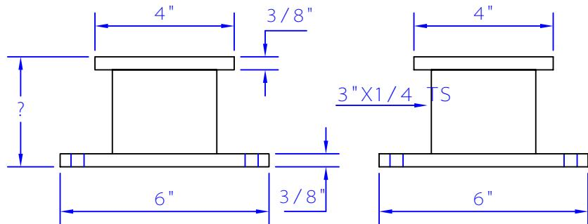
ALL FASTENERS, STEEL AND WELDS MUST BE DETERMINED BY A STRUCTURAL ENGINEER
